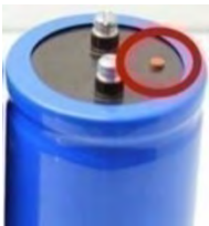
Figure 2— Fused Electrolytic Capacitor
